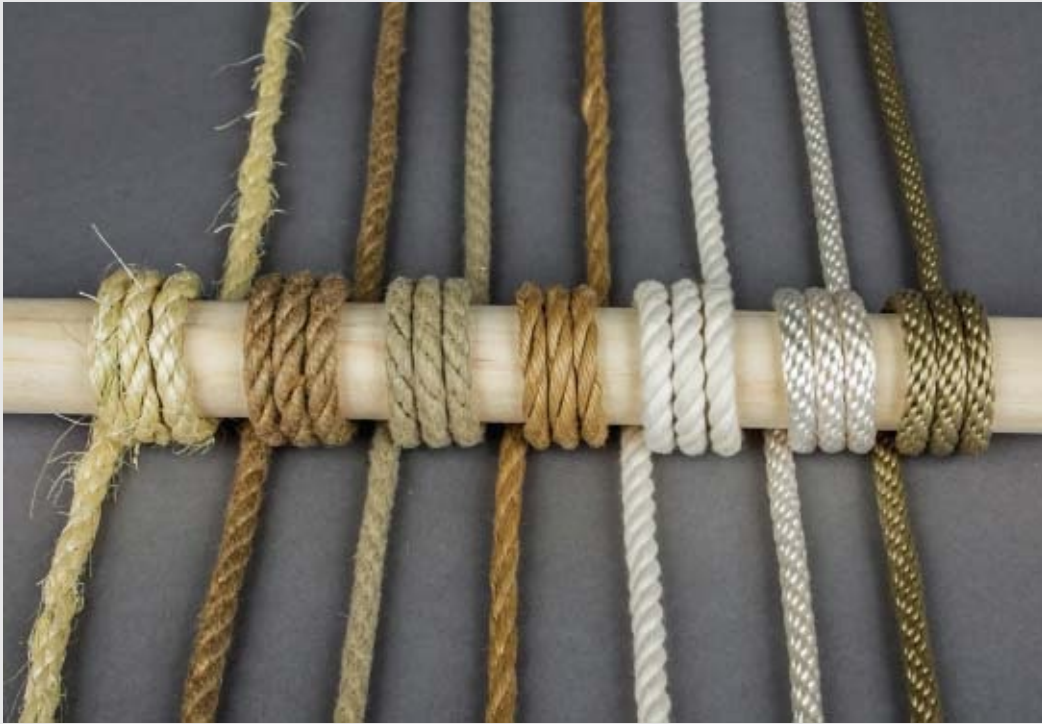
(From left to right) Sisal, Jute, Western Hemp, Japanese Hemp, Cotton, Nylon, Multifilament Polypropylene (MFP)
